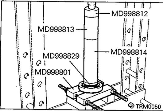
**HINWEISE ZUR MONTAGE****▶A◀ KUGELLAGER EINBAUEN**
